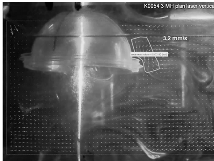
Figure D2. Vertical PIV—mean velocity magnitude in a selected area (vector scale 20)
